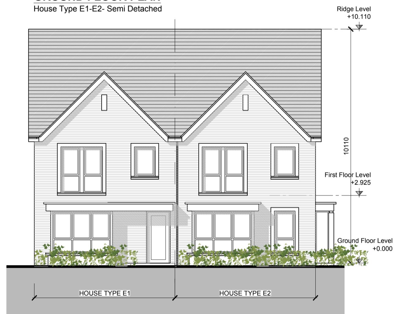
FRONT ELEVATION House Type E1-E2- Semi Detached
