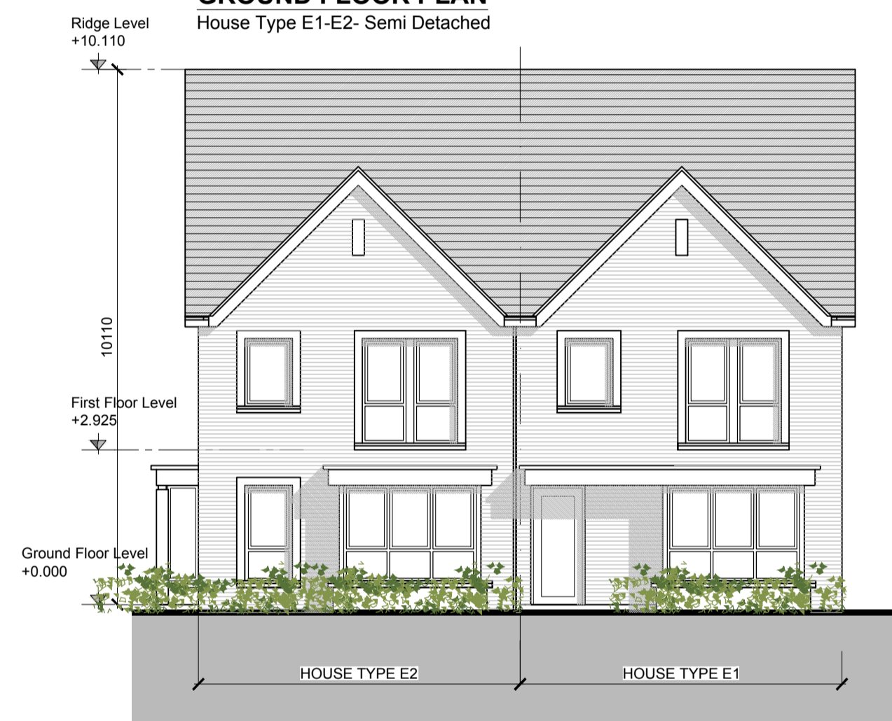
FRONT ELEVATION House Type E1-E2- Semi Detached
