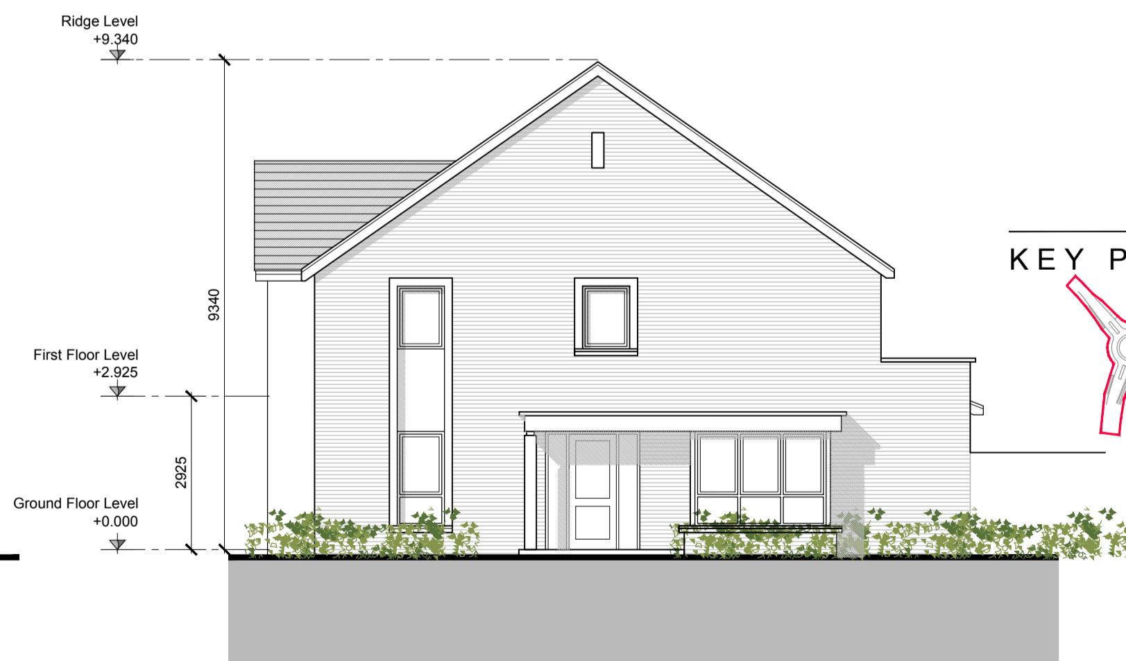
SIDE ELEVATION RIGHT Terrace Unit A2
